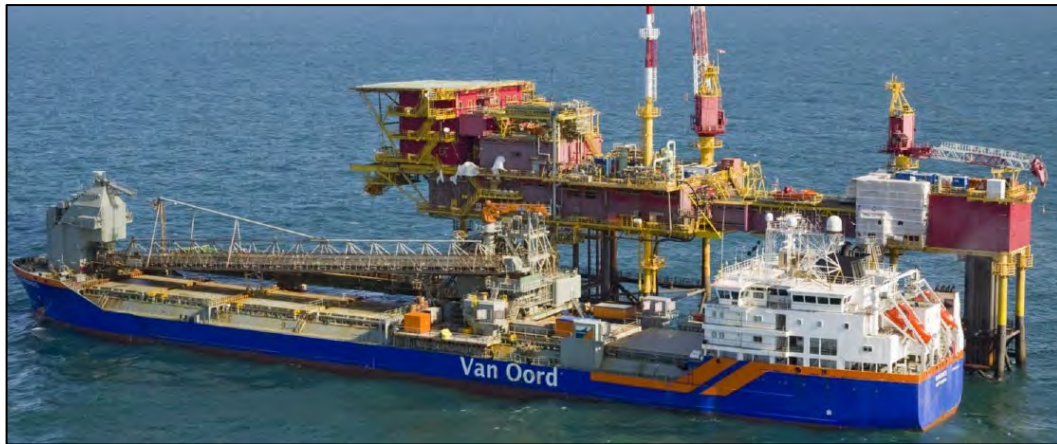
Figure B.5 – Rock Installation Vessel (Van Oord)
