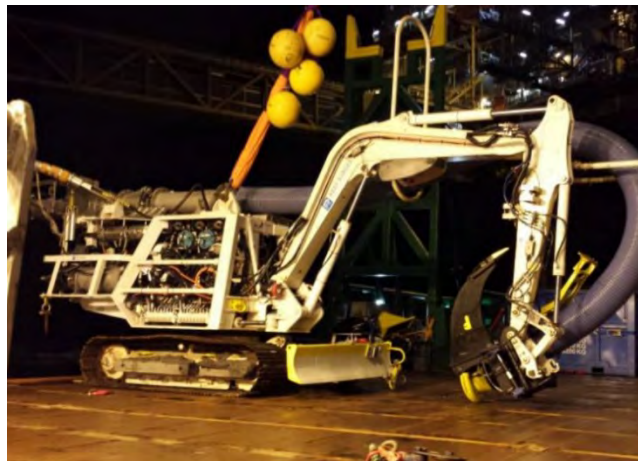
Figure B.11 – Subsea Excavator on Deck (Scanmachine)
