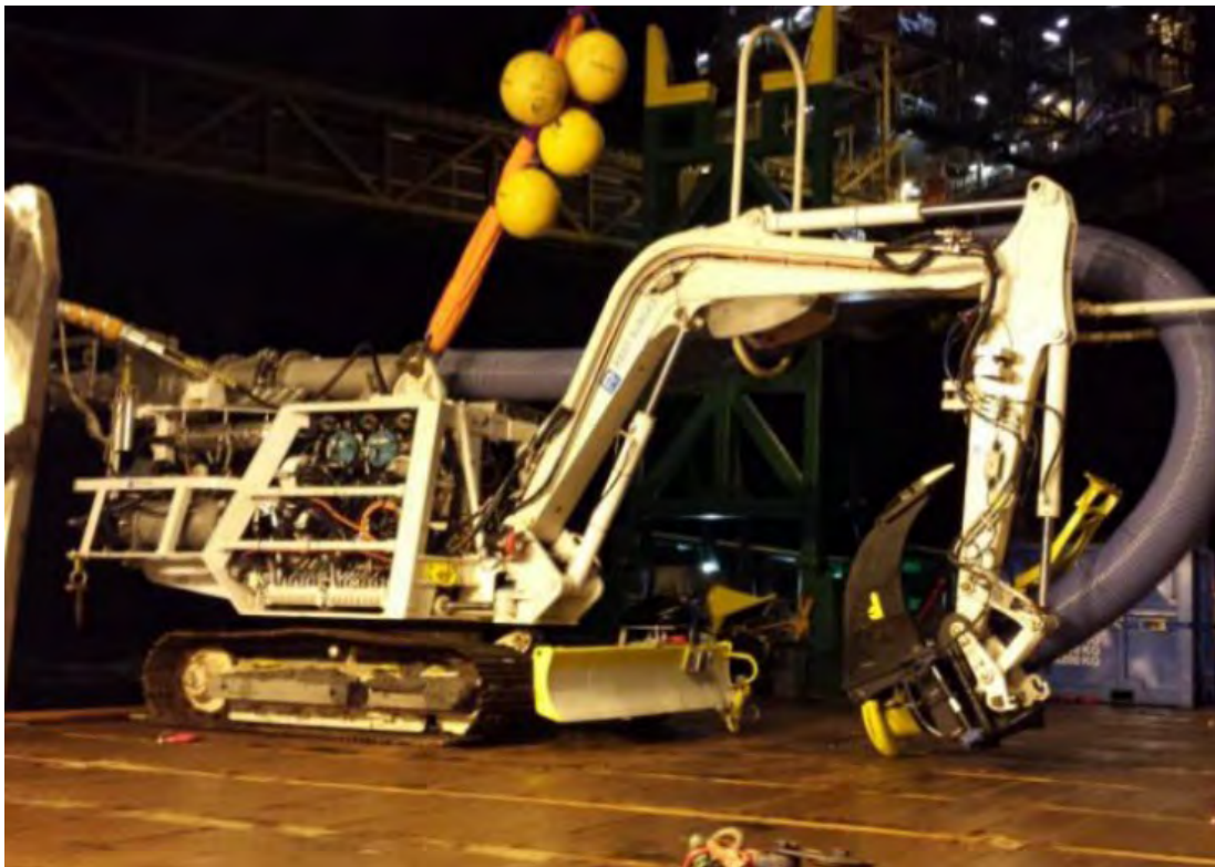
Figure 3-7 Seabed Excavator on Deck (Scanmachine)
