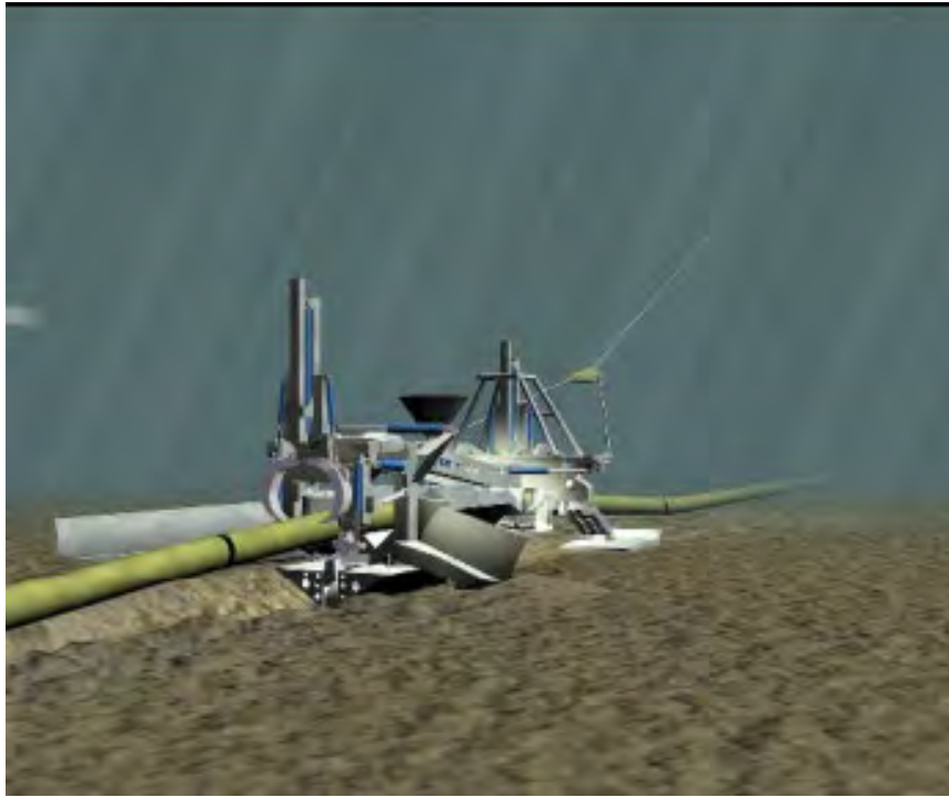
Figure B.18 – Ploughing with VMP
